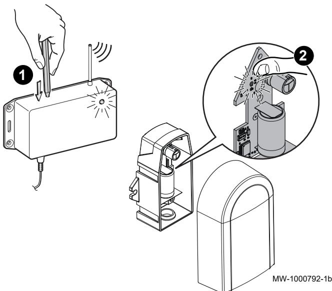
Each outside temperature sensor is given a unique identifying number in the factory, which enables the radio module to recognise it. This identifying number is transmitted to the radio module by the pairing sequence described below.
