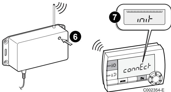
**6** **7** After a few seconds, the light on the radio module goes off and the remote control displays the message "init" while it synchronises itself with the module.
